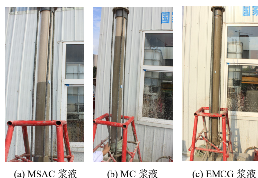
图6 MSAC、MC与EMCG浆液细砂层渗透扩散结果 Fig.6 Penetration grouting diffusion results for MSAC, MC and EMCG suspensions in fine sands
